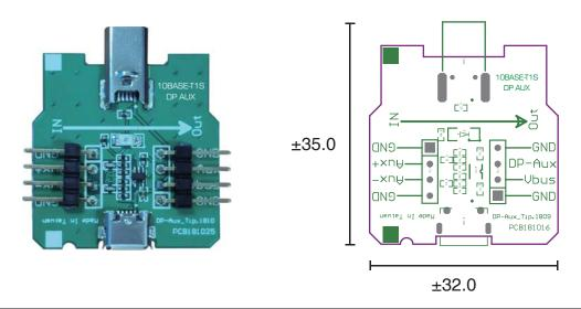
Convert differential signals to single-ended for 10BASE-T1S, facilitating signal analysis with a logic analyzer.
