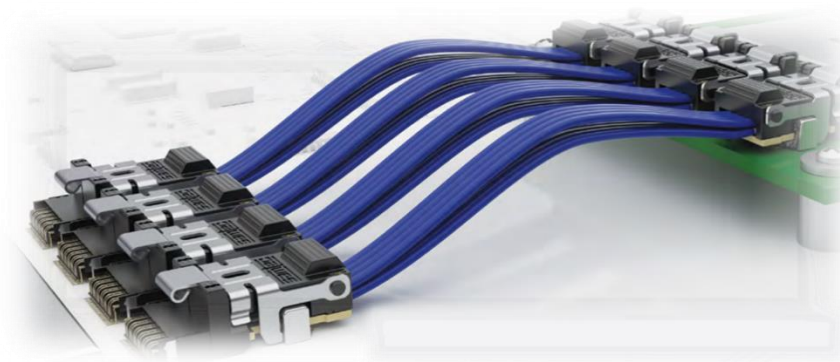
Figure 9 Conceptual illustration of the FireFly micro flyover system
