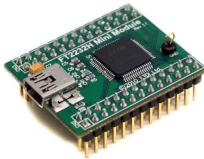
Figure 6 Illustration of the FT2232H USB-to-SPI converter module
