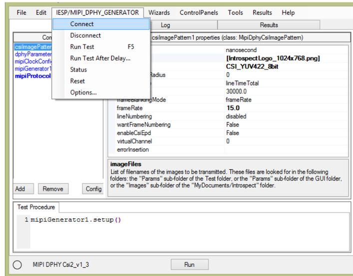
b. To verify the connection, select the pull-down menu "IESP/MIPI\_DPHY\_GENERATOR ->Status" three lines below the "Connect" entry, as shown above. A dialog window, as below, should confirm that the SV4D module is connected. The personality / firmware version may be more recent than the version shown below.
