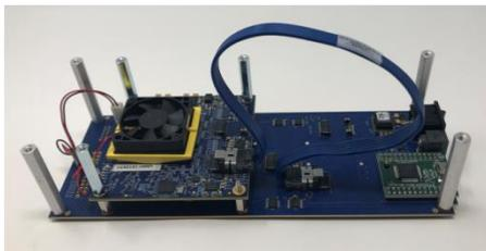
**Connect TX Port A (J35/36) of SV4D to J1/J2 of SV4M via Firefly Cable on underside of SV4M, as shown**
