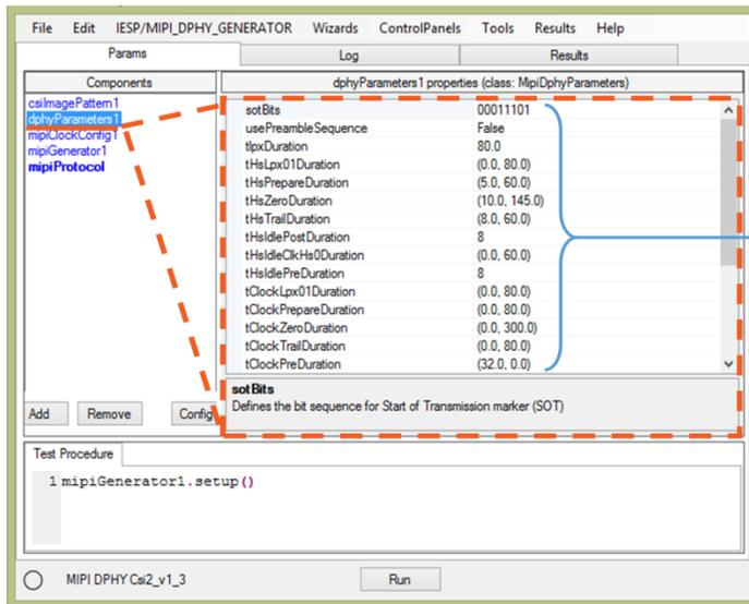
Global timing parameters are included in units of UI and nanoseconds exactly like the MIPI specification. SOT bits configurable on the fly for the purpose of testing.
