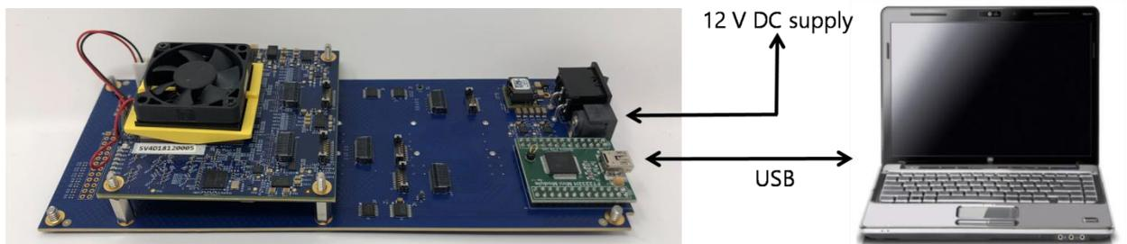
Figure 4 Connection for the automated FTDI driver installation.
