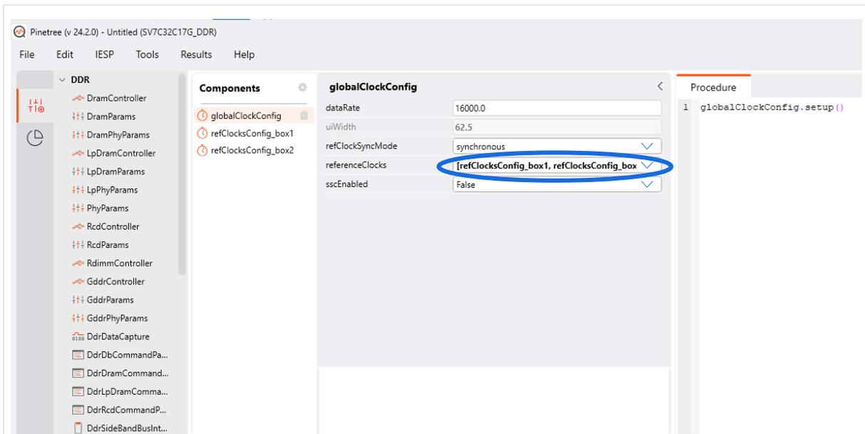
Figure 5: Screen capture showing two “referenceClocksConfig” components automatically created.
