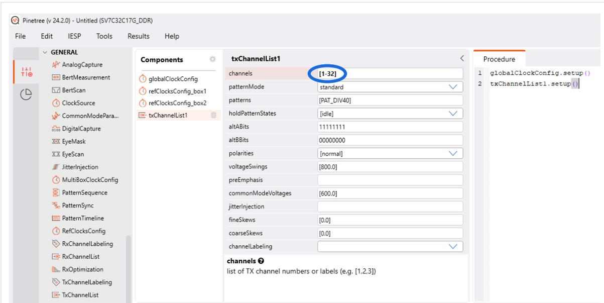
Figure 6: Changing the number of channels to the full range of 1-32.
