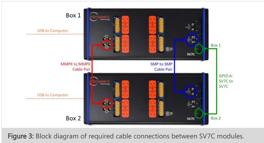
Figure 3: Block diagram of required cable connections between SV7C modules.
