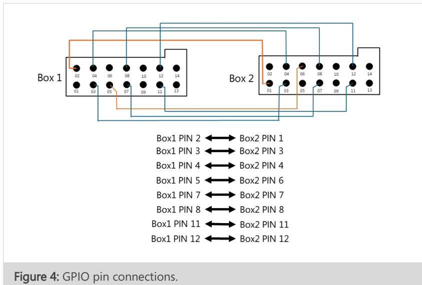
Figure 4: GPIO pin connections.
