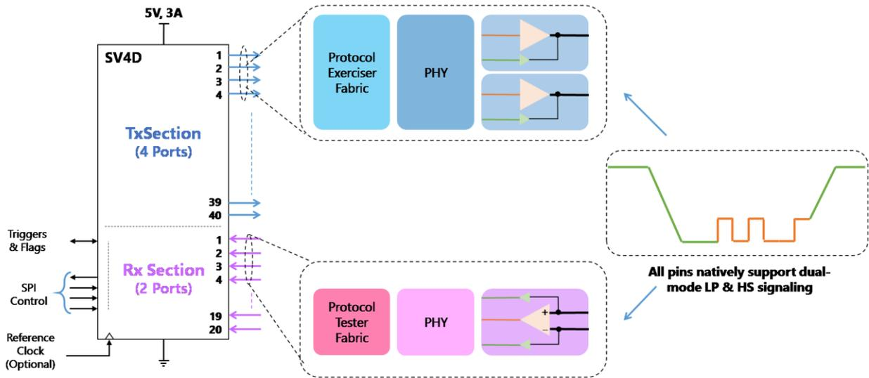
Figure 1 High level block diagram of the SV4D MIPI Test Module
