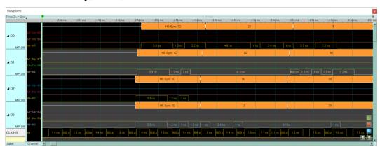
Ex: The width of high pulse in Lane 0, Lane 3 is not the width of half CLK cycle Half CLK cycle = (1.4 + 0.8) / 2 = 1.1 (ns)
