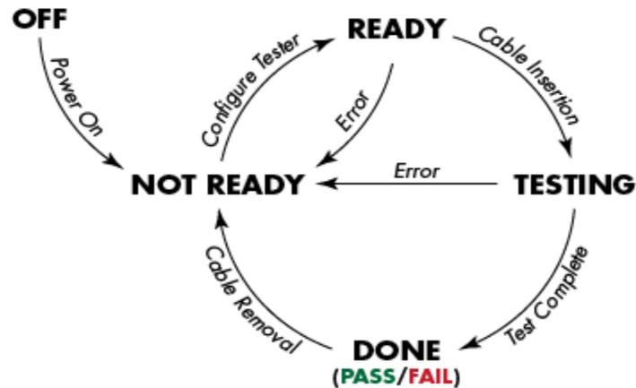
**Figure 11** : Advanced Cable Tester v2 Operational State Diagram
