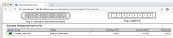
**Figure 35 :** Web Application - Individual Test Report - Source Measurement Unit Section
