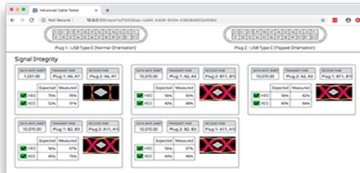
**Figure 31** : Web Application - Individual Test Report - Signal Integrity Section
