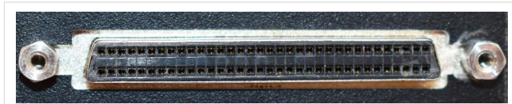
Figure 9: Photograph of the auxiliary control port on the SV1C
