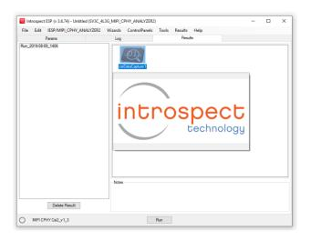
e) As can be seen, the SV3C-CPRX module was able to properly capture the Introspect Technology logo encoded using the CSI-2 protocol and transmitted over a single C-PHY lane.
