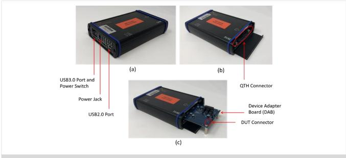
Figure 1: SV4E-DPTXCPTX connectors: (a) left side (b) right side (c) typical DAB connection
