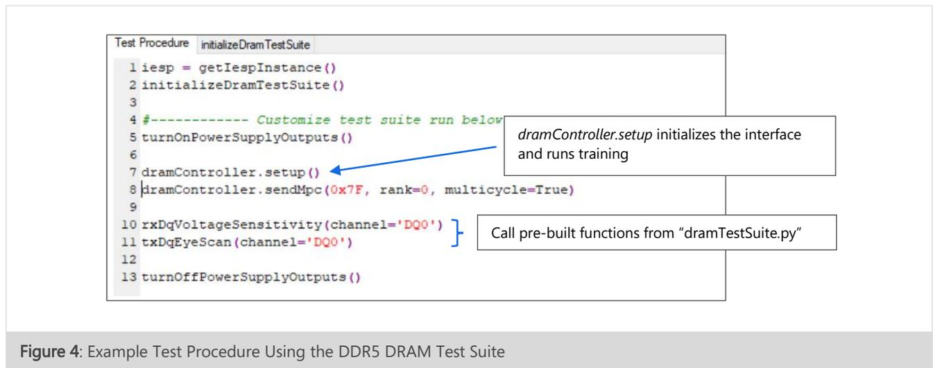
Figure 4: Example Test Procedure Using the DDR5 DRAM Test Suite
