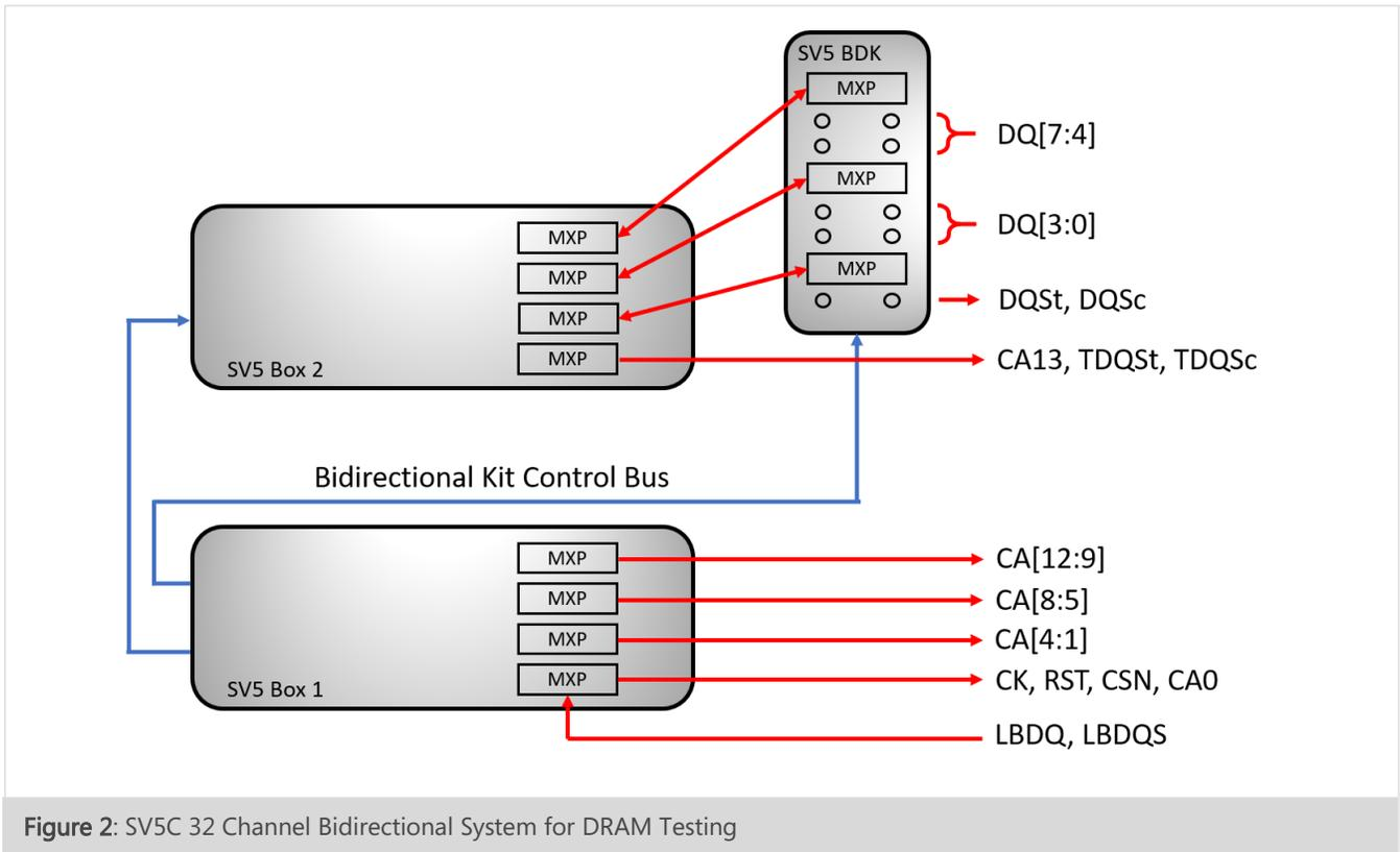
Figure 2: SV5C 32 Channel Bidirectional System for DRAM Testing
