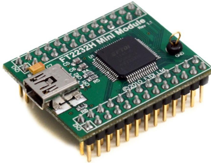
Figure 5 Illustration of the FT2232H USB-to-SPI converter module.
