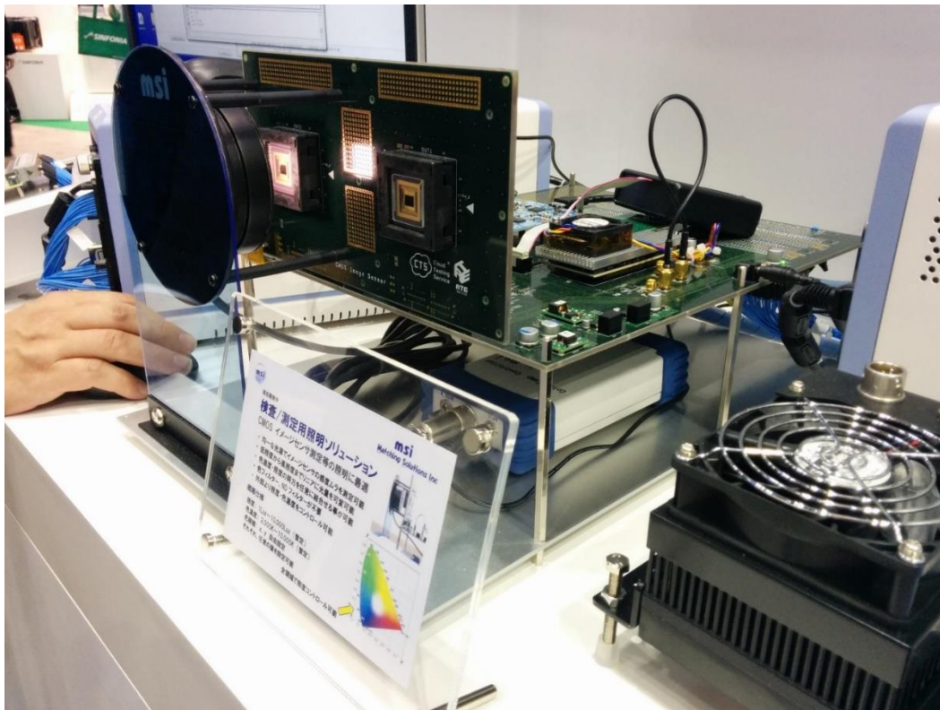
Figure 13 Illustration of a complete protocol-based image sensor test system based on Introspect's SV1D plug-in test card.
