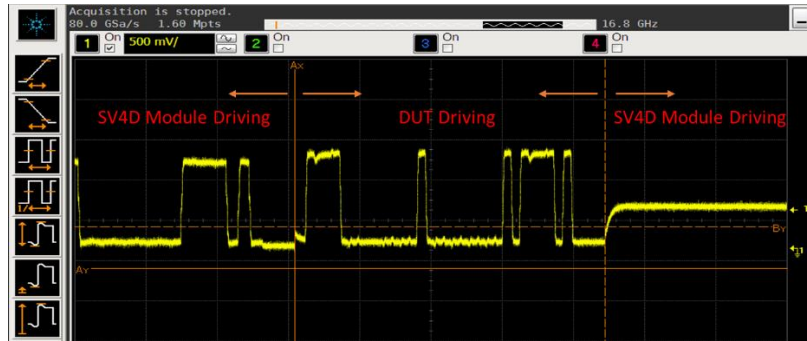
Figure 8: Bus turnaround waveform from an actual device test sequence
