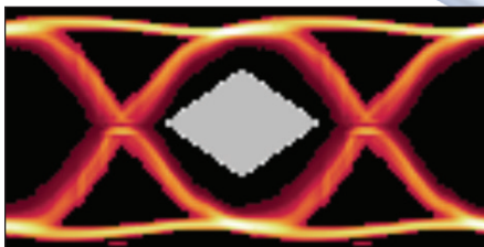
Passing eye-diagram 10 Gbps USB Type-C to USB Type-C cable.
