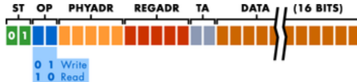
Figure 27 : Basic MDIO Frame Format
