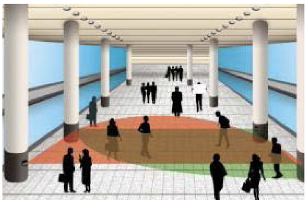
Adjusting air-conditioning and lighting depending on the density of people for energy saving
