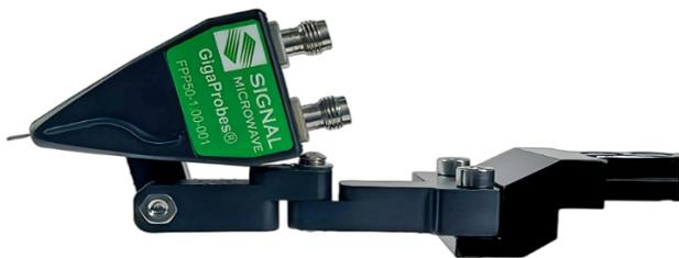
Vertical 90° Probing: Probe horizontally oriented test pads on a vertically fixtured PCB
