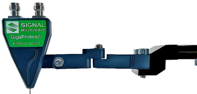
Vertical Probing: Probe Vertically oriented test pads on a vertically fixtured PCB
