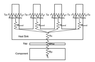
Figure 4. Electrical Package and Heat Sink Thermal Resistance.
