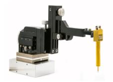
Rigid arm probe manipulator with XYZ pitch 40 TPI controls & magnetic base. Recommended for probing with DVT40 and DVT-FPPXX probes.
