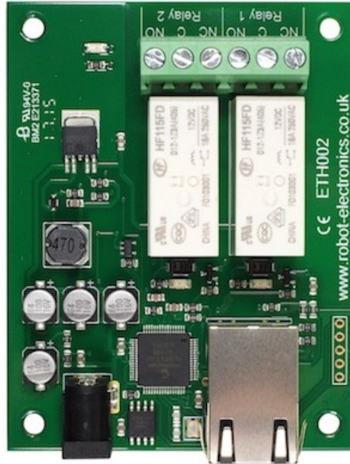
12v dc 2.1mm jack (+ve core) RJ45 Ethernet
