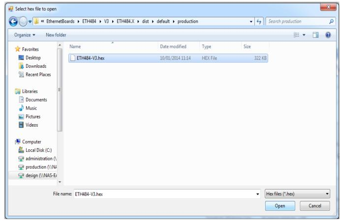
Once the file has been opened the programming sequence will now begin, it's fairly short and following it's completion the board will reset (automatically) and the LED will flash quickly while the programming sequence completes. Do not turn the power off in this sequence.
