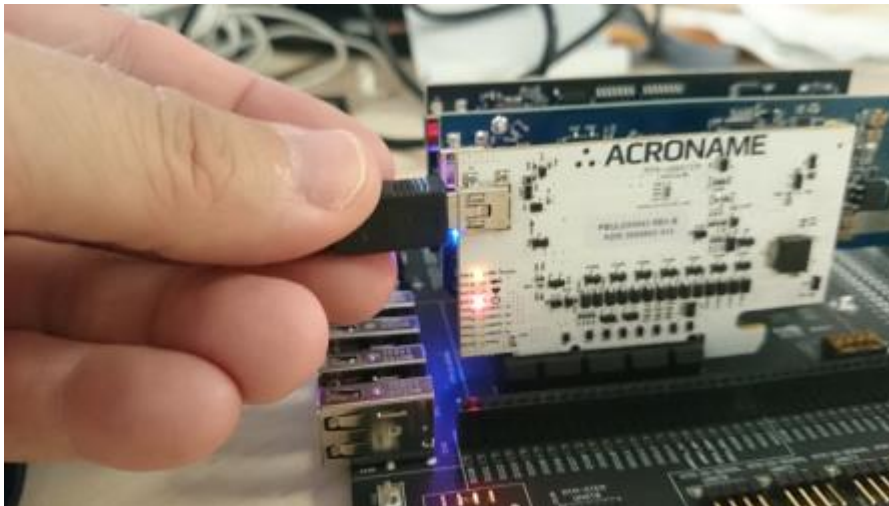
Figure 14: USB Host connection to the USBStem
