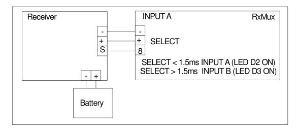
In this set-up, power to the RxMux will be provided via the Receiver. Configure your transmitter to send a servo signal less than 1.5ms wide. LED D1 should be off indicating a valid select signal is being received. LED D2 will turn on indicating Input A is selected. Next, configure you transmitter to send a servo signal greater than 1.5ms wide. LED D3 will turn on indicating Input B is selected.
