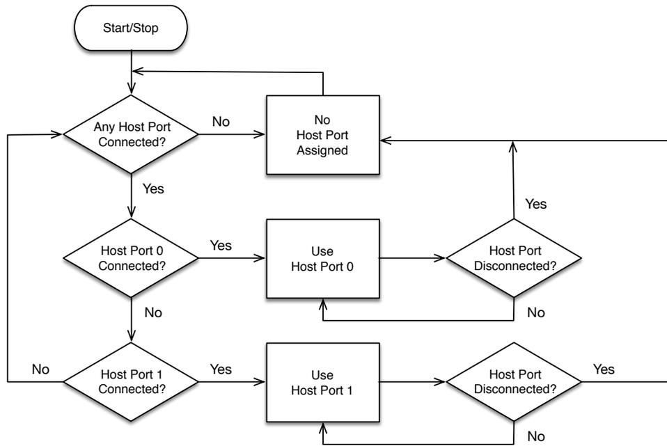
Figure 6: Determining connection used for BrainStem communications
