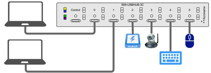
Testing multiple devices against different computer systems is easily done using AnyPort™ technology. Software control to select which port becomes an upstream facing port enables better regression systems and testing for product reliability.
