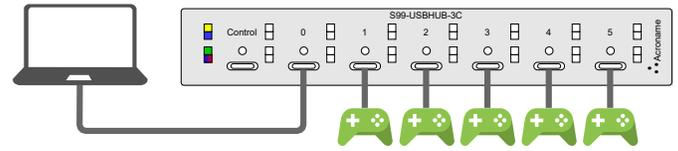
Charge and verify data connectivity and throughput. Verify PD negotiation with automated cable flip.
