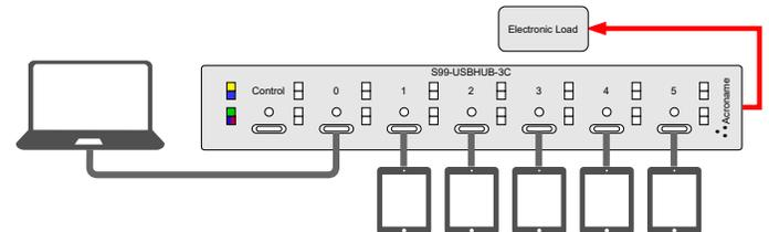
Automate data role swapping for validating products that can act as both a USB host and peripheral as well as a power source or sink through USB-PD protocol. USB-C Hub's Power Delivery negotiation can facilitate changes to a DUT's V<sub>bus</sub> exercisable with an electronic load.
