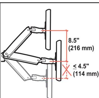
EN \* The lower most range of motion for vertical lift is decreased up to 4.5" (114 mm) when arm is adjusted to hold over 20lbs (9 kgs).
