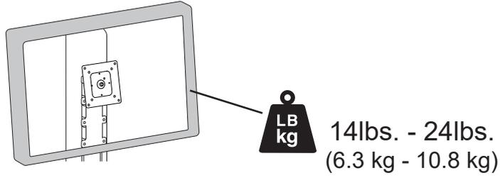
Total weight of monitor when mounted needs to be 14 lbs - 24 lbs (6.3 kg - 10.8 kg)
