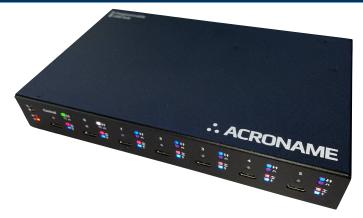
The **USBHub3c** from Acroname® is the world's first and only programmable USB Type-C® hub. It can automate validation, control, and test the limits of devices built on the Power Delivery (USB-PD) and USB specification. Simple software APIs allow control over all USB-PD modes and parameters, including intentional error states, connectivity options and real time measurements.
