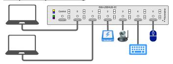
Testing multiple devices against different computer systems is easily done using AnyPort™ technology. Software control to select which port becomes an upstream facing port enables better regression systems and testing for product reliability.
